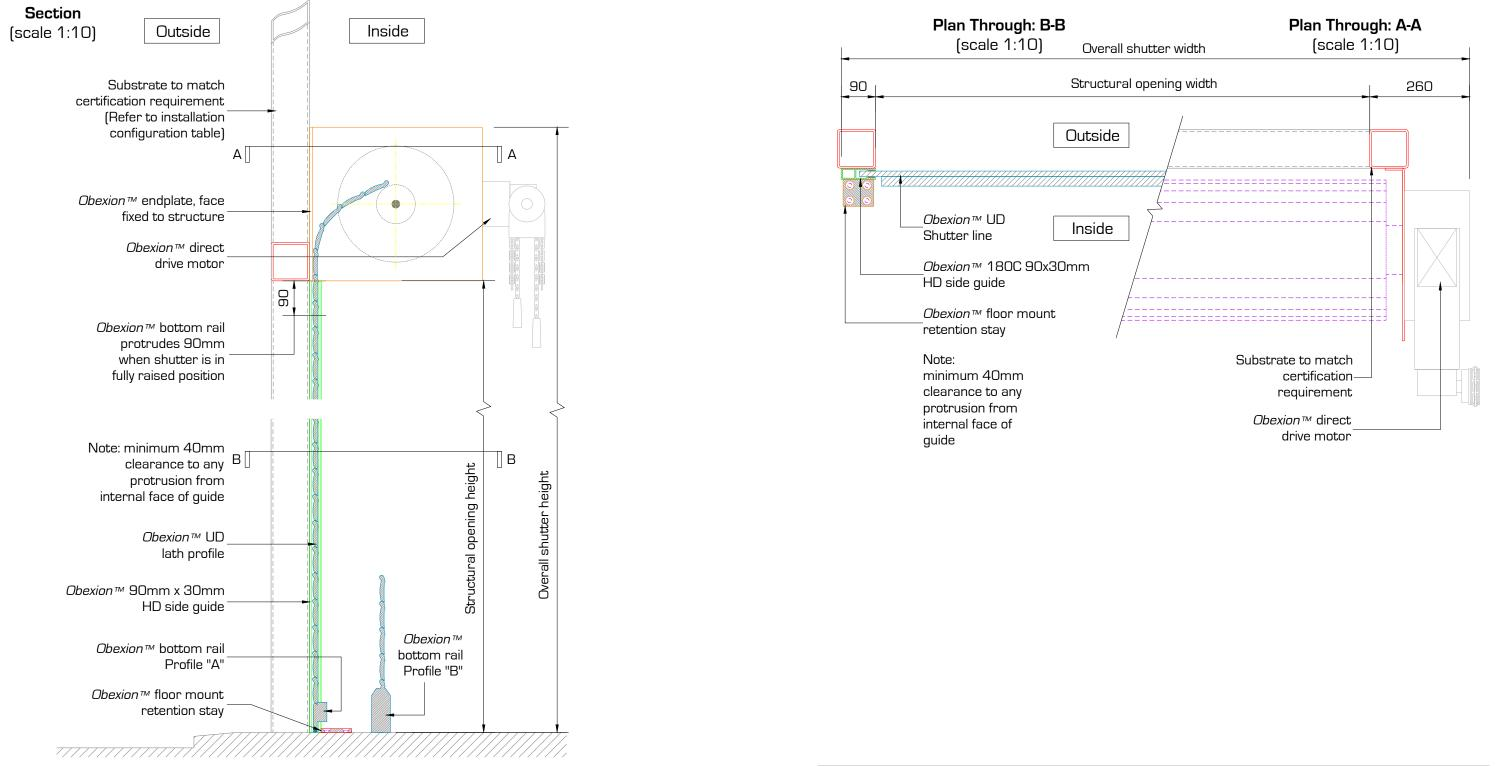
NOTE: The installation shall be direct to the substrate and not via intermediate substrates, such as plasterboard
